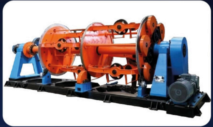
Core Laying-up Machine
